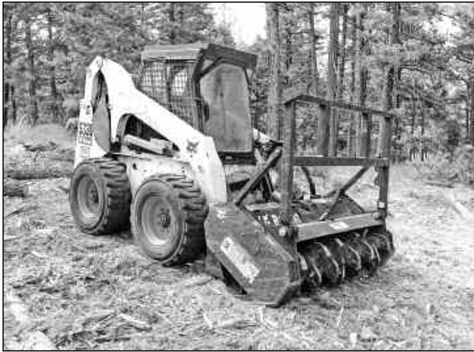
A masticator was used to remove the trees on Tincup to create a fuel break.
